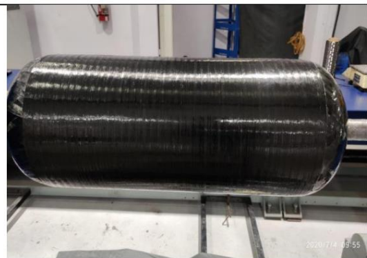
Figure: Type-IV H 2 Pressure vessel
