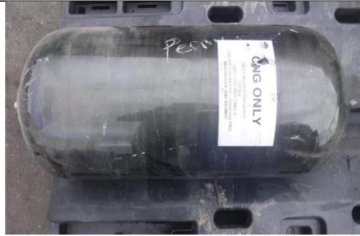
Figure: Type-IV CNG Pressure vessel
