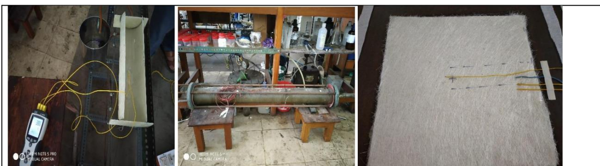
Figure: FBG Sensor based smart composite pipe
