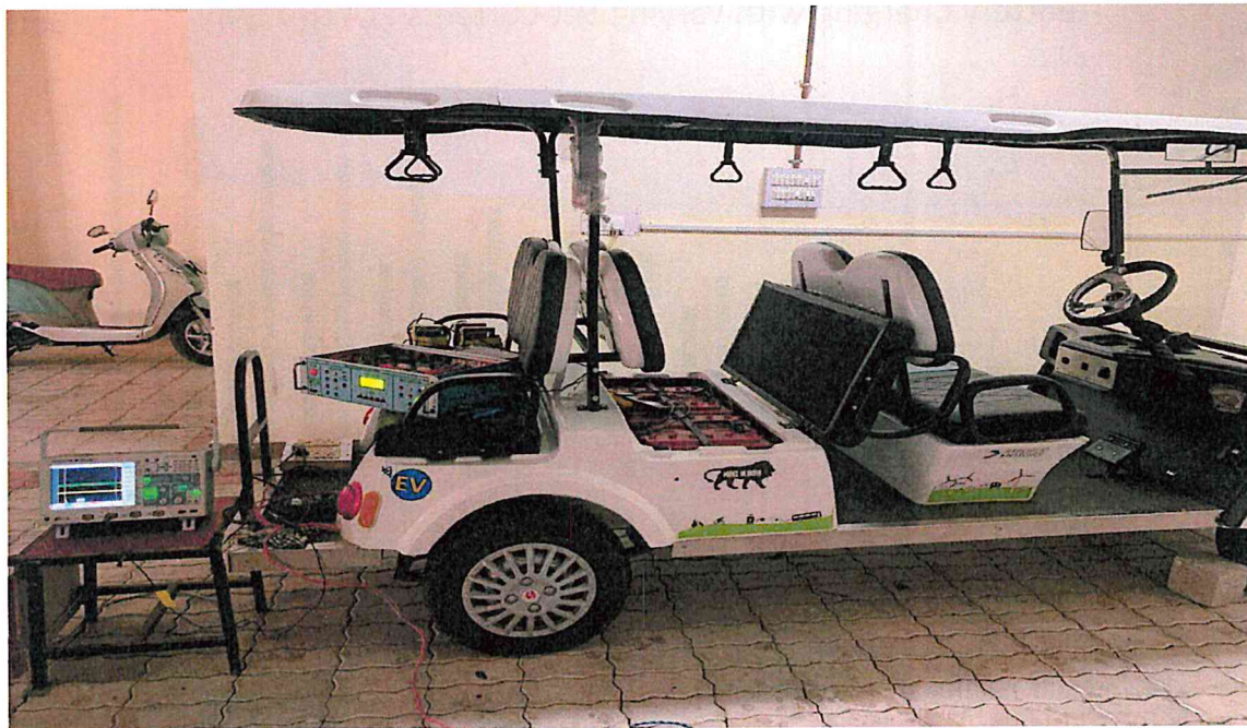
Fig. 11: Testing setup for a high-frequency transformer-based EV charger
