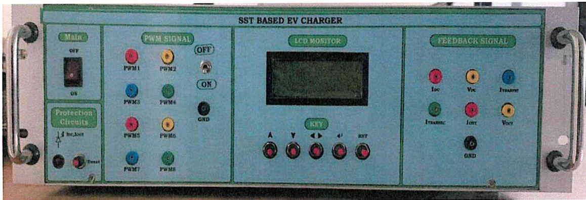
Fig 4: SST based EV charger
