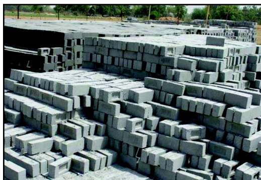
Figure A3.10. Fly Ash Bricks Image
